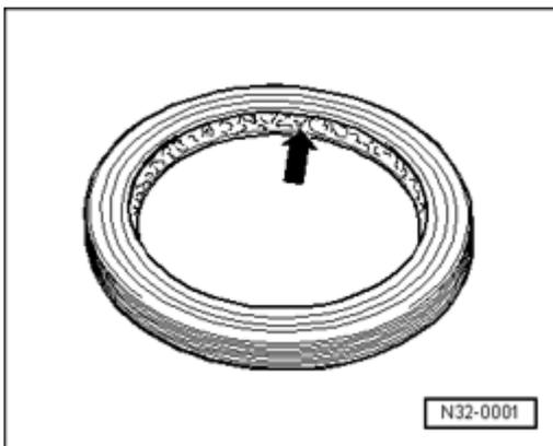
**Fig. 5: Identifying Space Between Oil Seal Sealing Lips**
