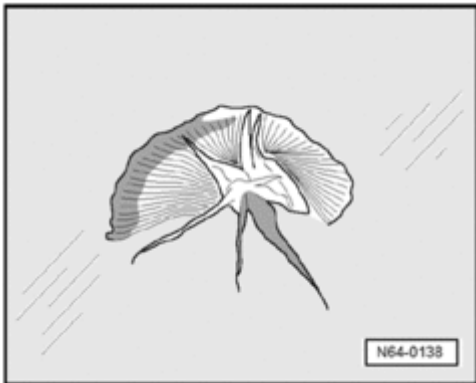
Fig. 37: Identifying Star And Crack Damage Courtesy of VOLKSWAGEN UNITED STATES, INC.
