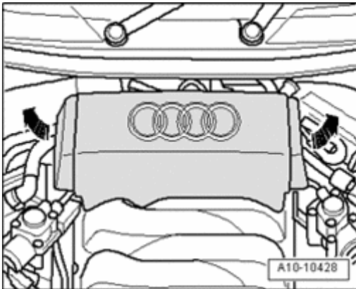
Fig. 562: Removing Rear Engine Cover
