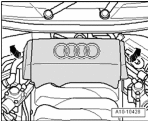
Fig. 590: Removing Rear Engine Cover
