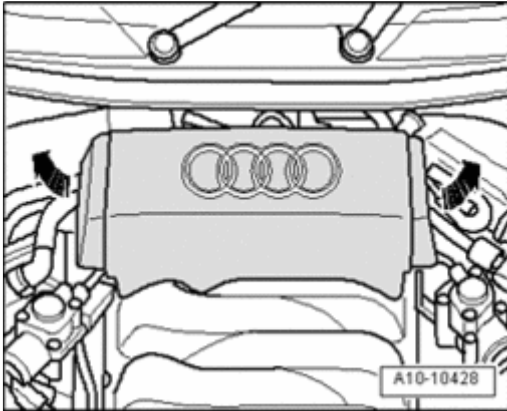
Fig. 592: Removing Rear Engine Cover
