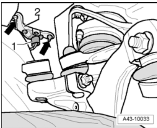
Fig. 472: Identifying Connector, Nuts, And Body Acceleration Sensor Courtesy of VOLKSWAGEN UNITED STATES, INC.
