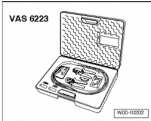
Fig. 157: Fiber Optic Plier Repair Set VAS 6223 Courtesy of VOLKSWAGEN UNITED STATES, INC.
