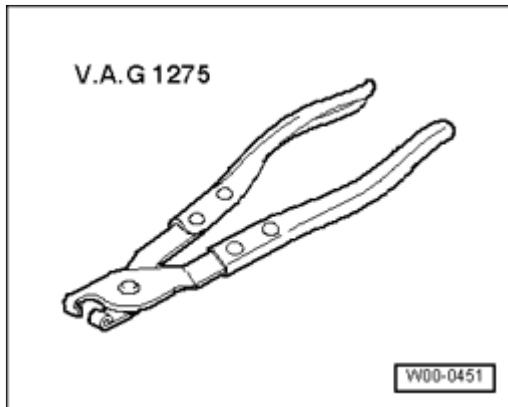
Fig. 197: Identifying Hose Clamp Pliers V.A.G 1275 Courtesy of VOLKSWAGEN UNITED STATES, INC.
