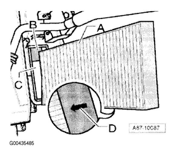
Fig. 3: Removing/Installing Dust & Pollen Filters Courtesy of AUDI OF AMERICA, INC.
