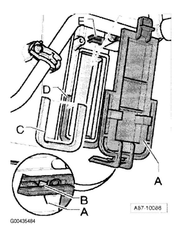
Fig. 2: Removing/Installing Dust & Pollen Filter Cover Courtesy of AUDI OF AMERICA, INC.
